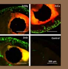
shaft from Zn-1Mg, Zn-1Ca, Zn-1Sr implanted pins groups and the sham control group observed under fluorescent microscopy at week 8. The green fluorescence indicates the new bone formation.
